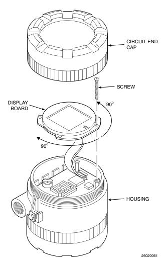
Figure 2-8. Display Positioning Assembly
